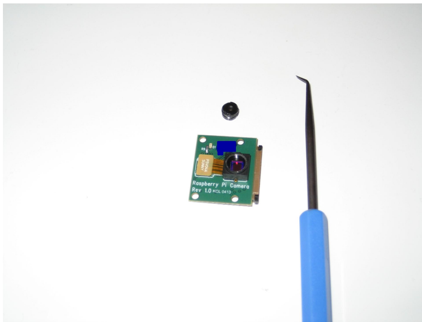
Figure 45: Removing Epoxy from Lens Assembly
